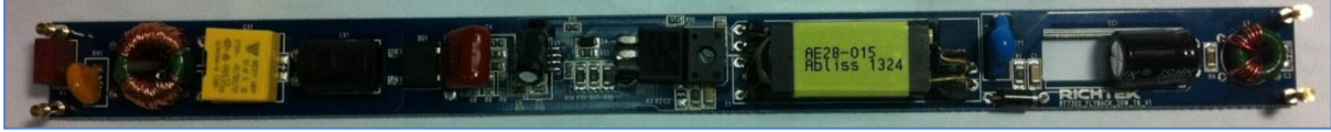
Figure 3. The board measures 230x18x10mm and will fit in most narrow tube T8 housing behind the LED board.
